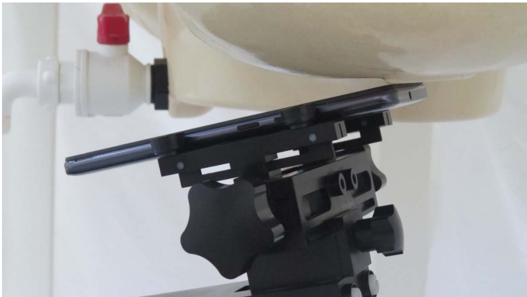
Picture 2: Left Hand Tilt 15 Degree Position
