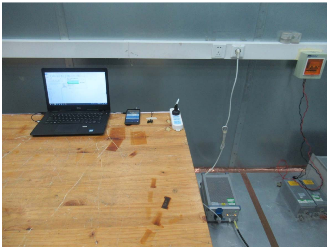
Picture 1: Conducted Emissions Test Setup
