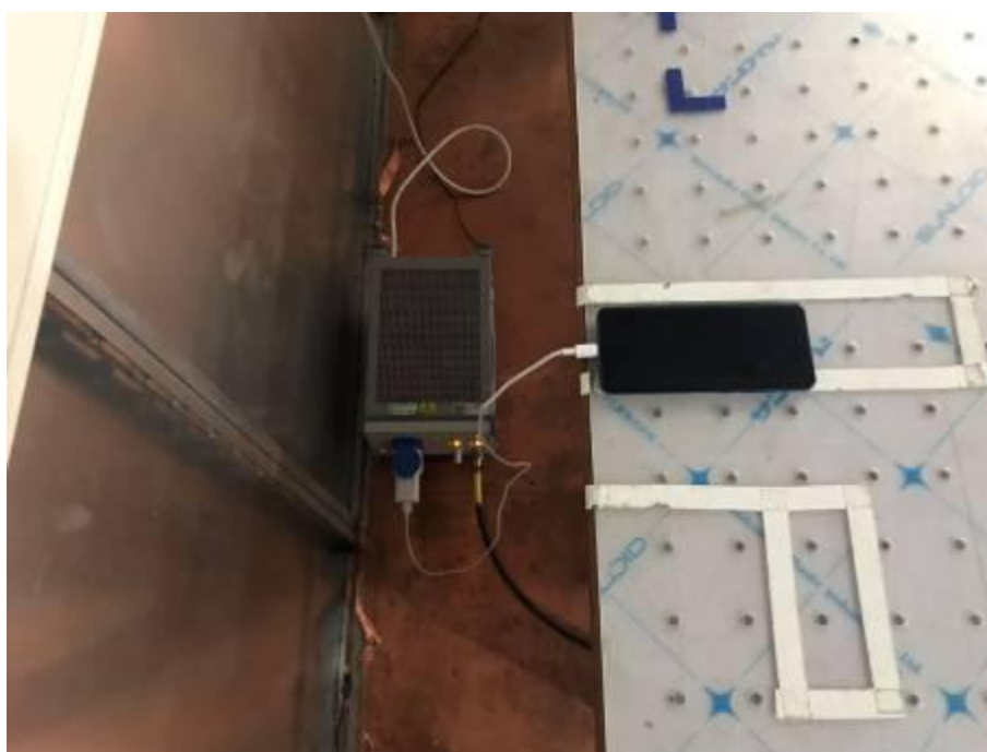
Conducted Emissions Test Setup (with charger)
