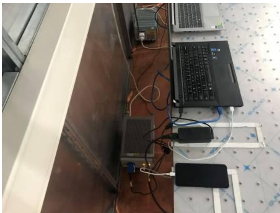
Conducted Emissions Test Setup (with laptop)
