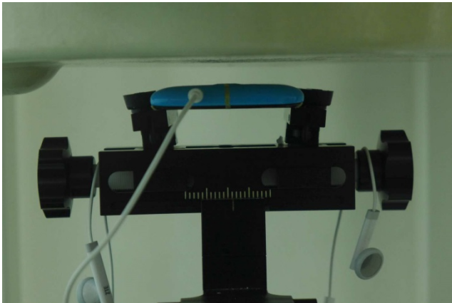
Back with Headset, Test Separation 1 cm
