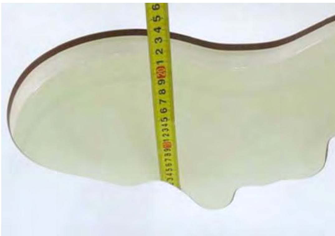
Picture 7: Liquid depth in the head Phantom (2600 MHz, 15.4cm depth)
