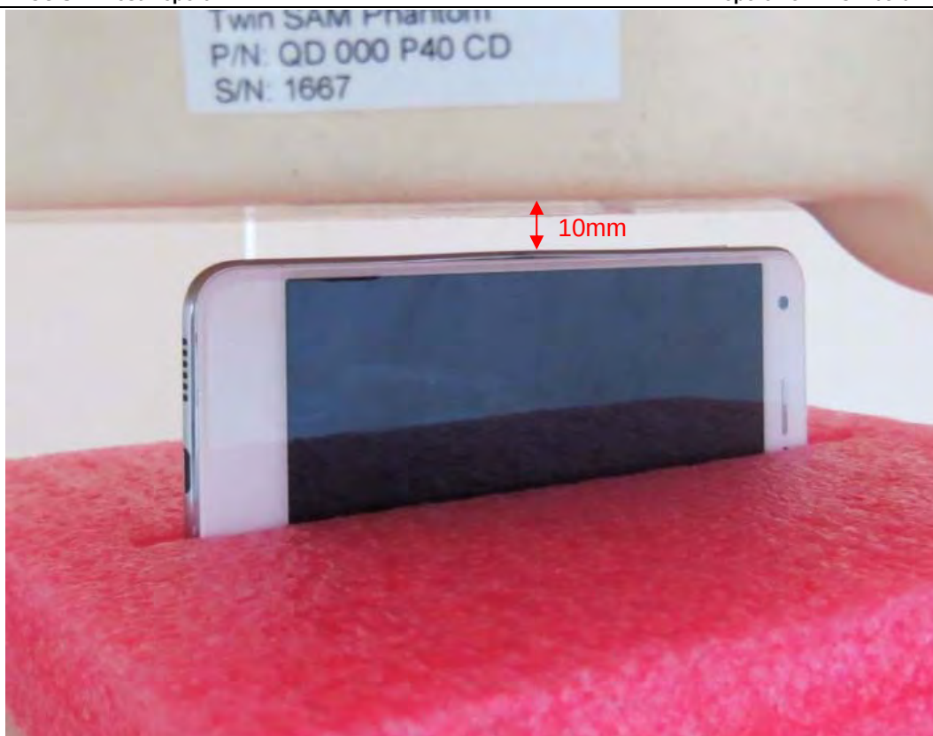
Picture 16: Left Side, the distance from handset to the bottom of the Phantom is 10mm
