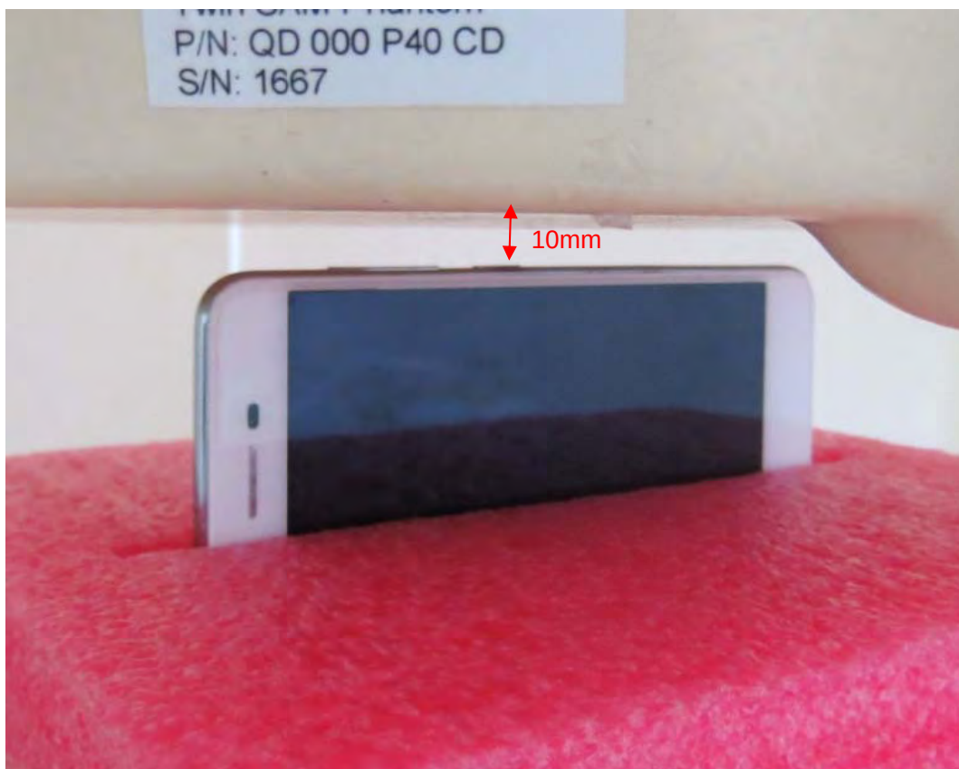
Picture 17: Right Side, the distance from handset to the bottom of the Phantom is 10mm
