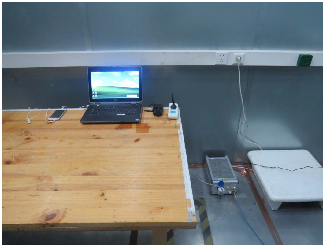
Picture 3 Conducted Emission Test Setup
