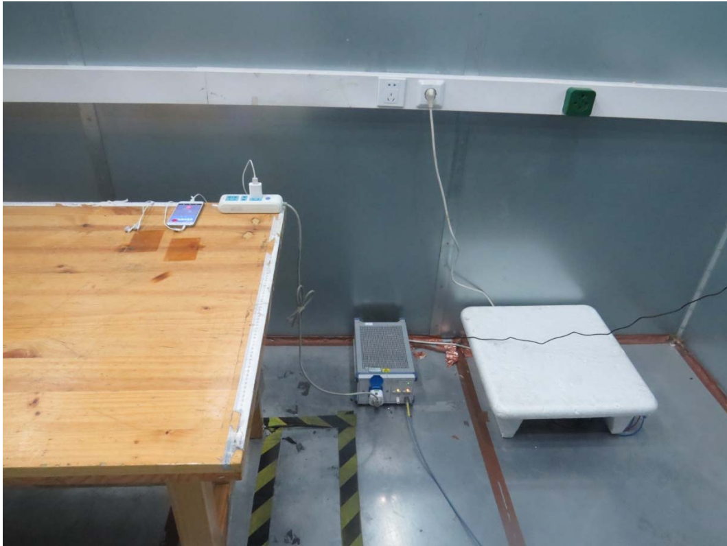
Picture 3 Conducted Emission Test Setup
