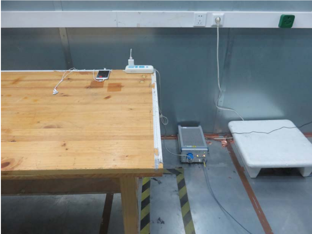
Picture 3 Conducted Emission Test Setup
