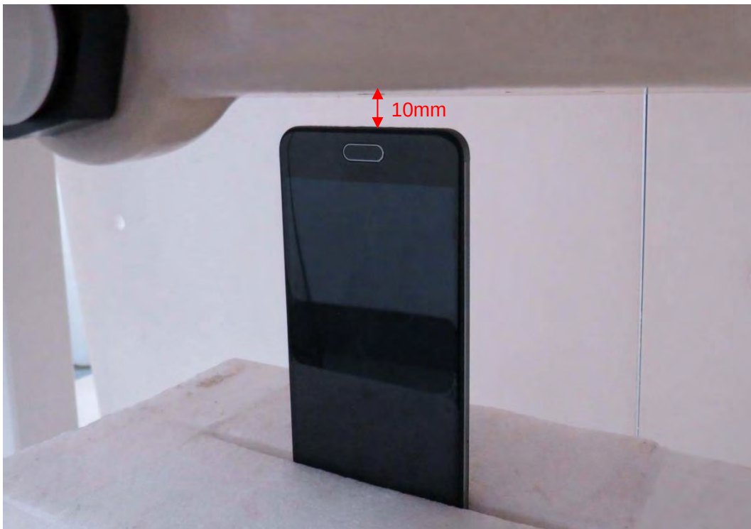
Picture 25: Bottom Side, the distance from handset to the bottom of the Phantom is 10mm
