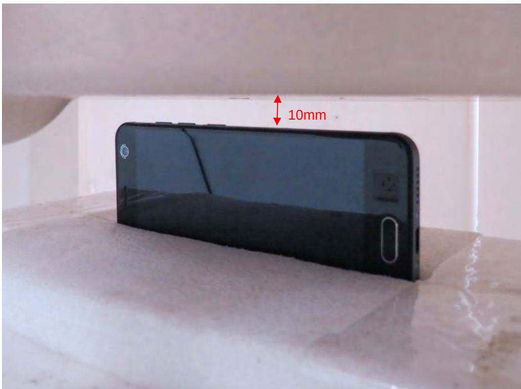
Picture 23: Right Side, the distance from handset to the bottom of the Phantom is 10mm
