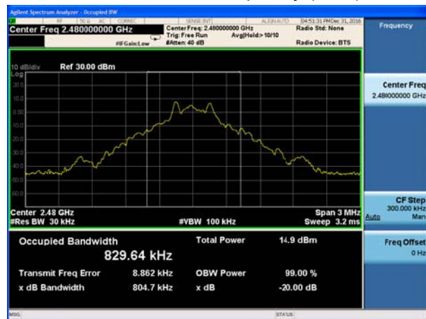
BT DH5 CH78, Carrier frequency (MHz): 2480
