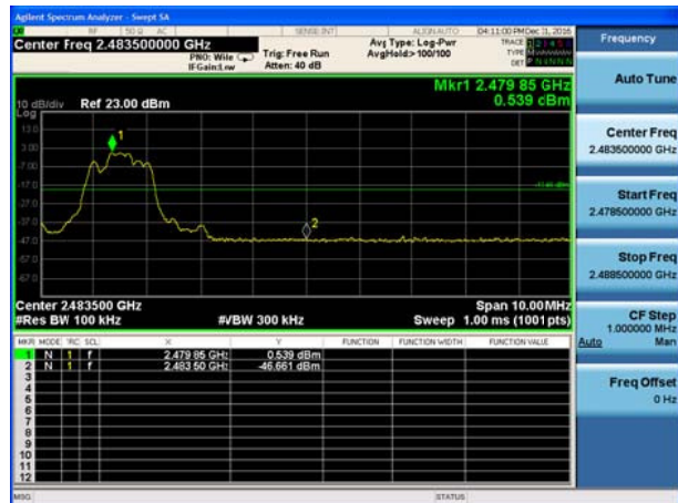
BT 3DH5 CH78, Carrier frequency (MHz): 2480
