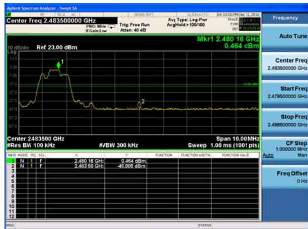
BT 3DH5 CH78, Carrier frequency (MHz): 2480
