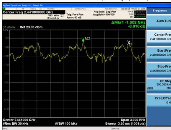
BT 2DH5 CH39, Carrier frequency (MHz): 2441
