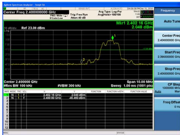
BT 3DH5 CH0, Carrier frequency (MHz): 2402
