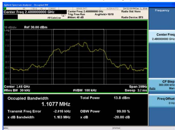
BT 2DH5 CH78, Carrier frequency (MHz): 2480
