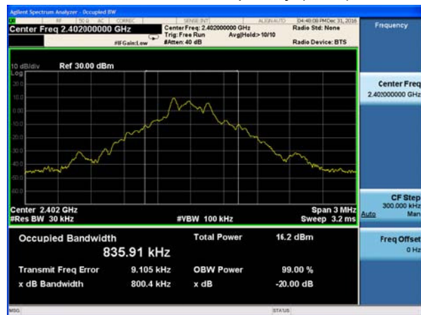
BT DH5 CH39, Carrier frequency (MHz): 2441
