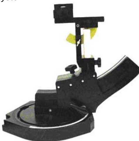
Device holder supplied by SPEAG
