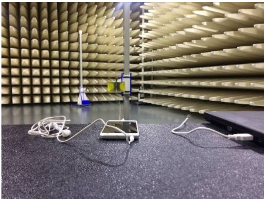
Radiated Emissions Test Setup (with laptop)
