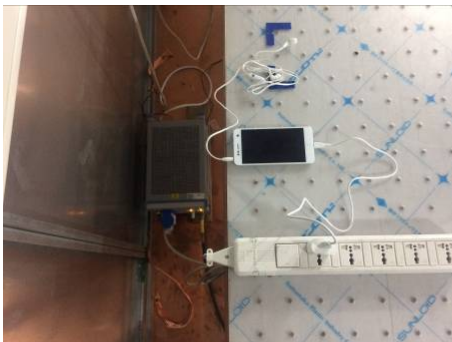
Conducted Emissions Test Setup (with charger)
