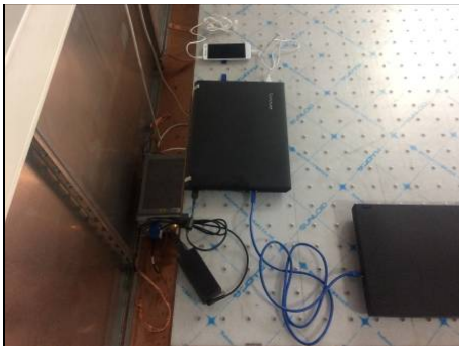
Pic8. Conducted Emissions Test Setup (with laptop)
