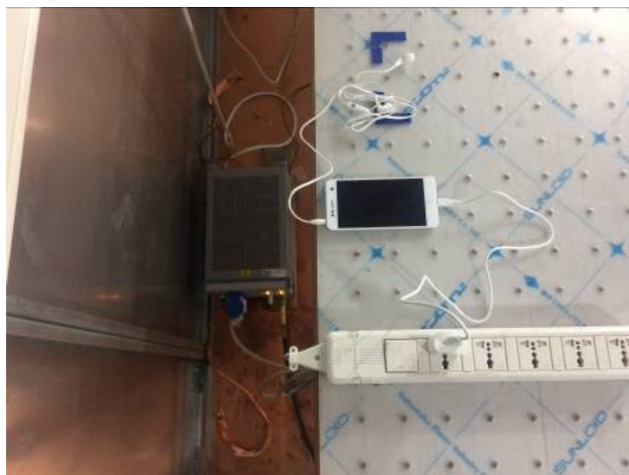
Pic9. Conducted Emissions Test Setup (with charger)
