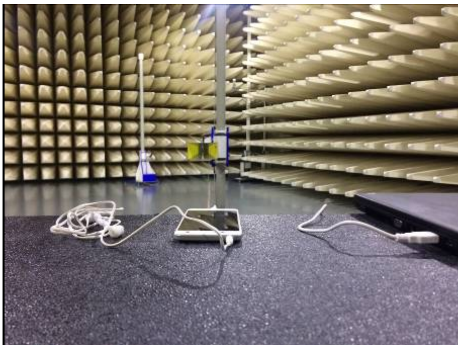
Pic6.Radiated Emissions Test Setup (with laptop)
