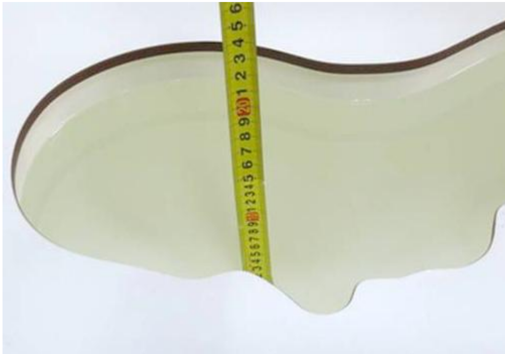
Picture C.9: liquid depth in the head Phantom (1750 MHz) (15.1cm deep)
