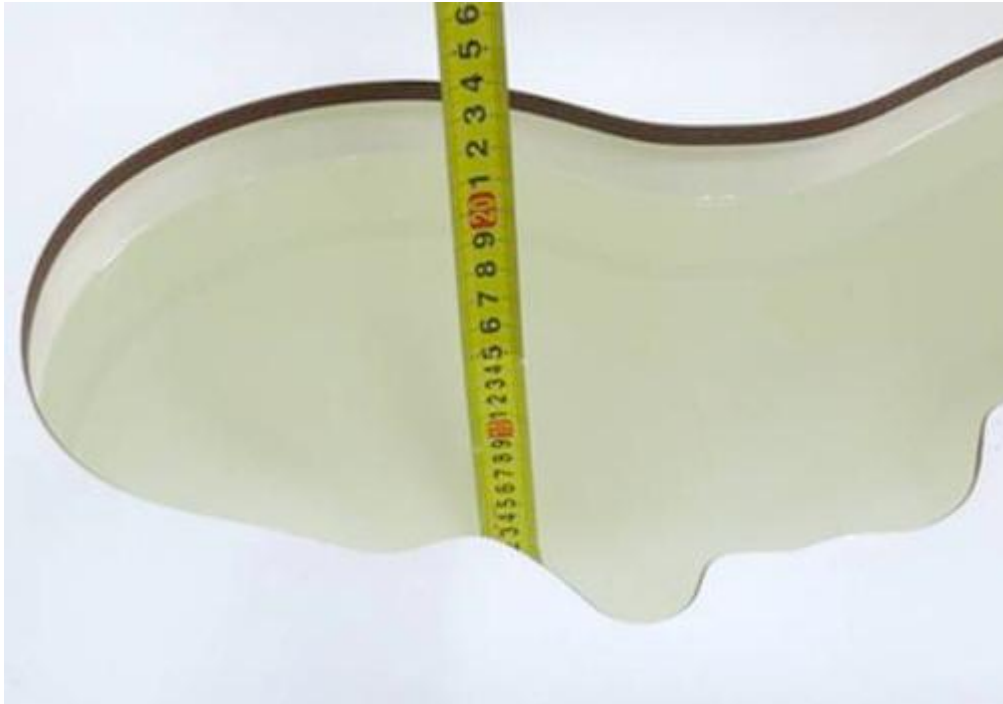
Picture C.5: liquid depth in the head Phantom (1900 MHz) (15.2cm deep)
