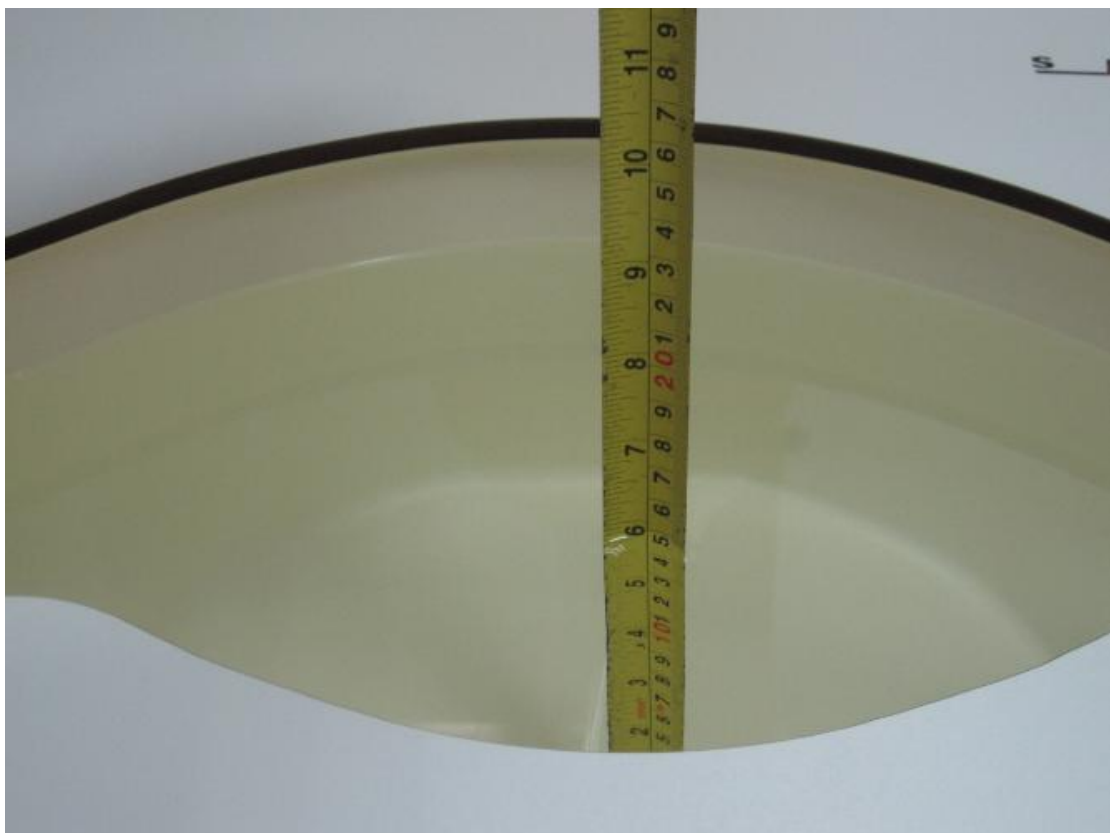
Picture C.4: Liquid depth in the flat Phantom (1900 MHz) (15.3cm deep)
