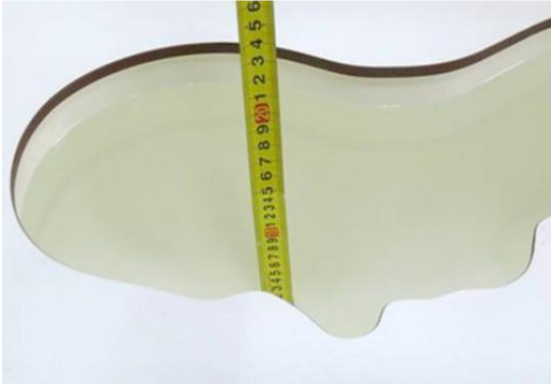
Picture C.7: liquid depth in the head Phantom (2450 MHz) (15.2cm deep)
