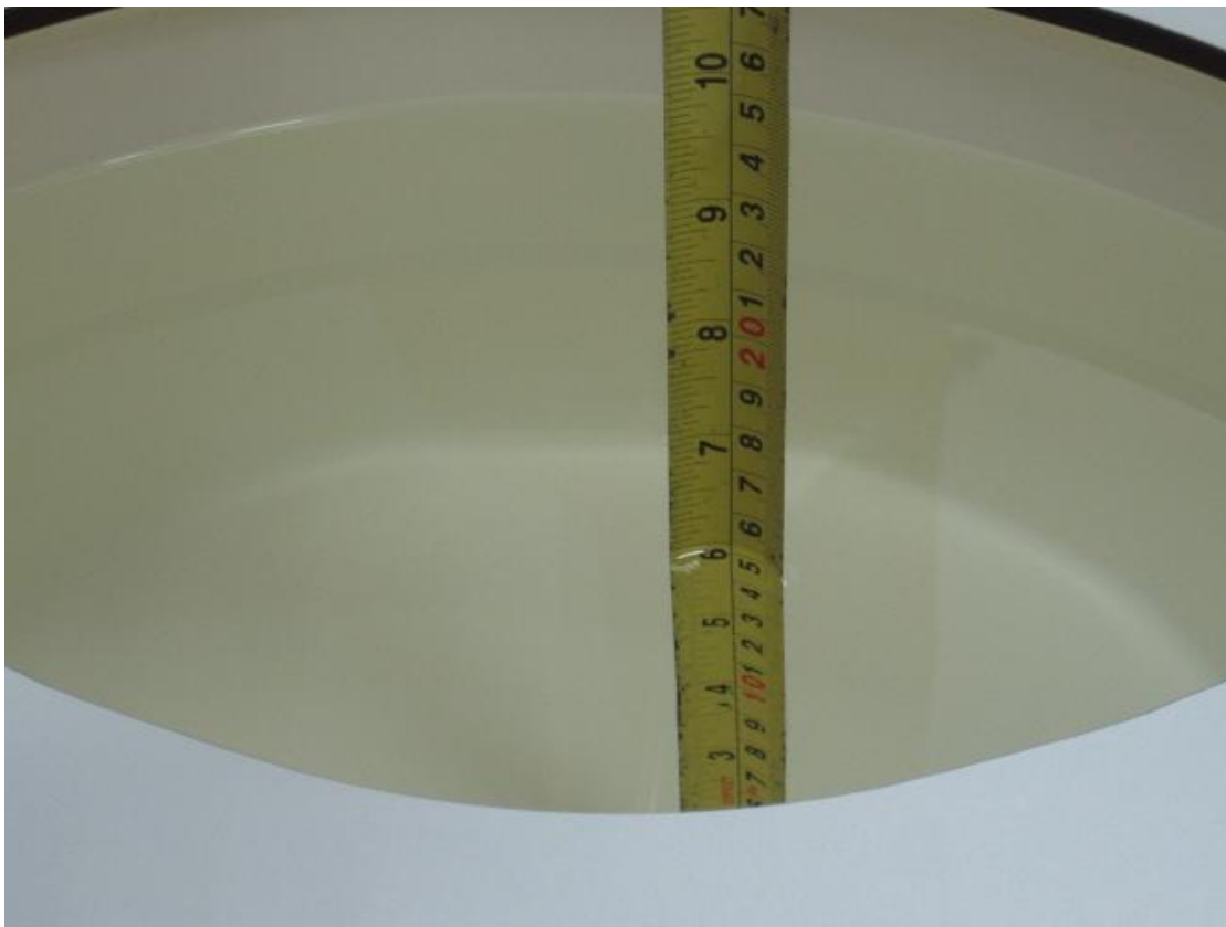
Picture C.8: Liquid depth in the flat Phantom (1750 MHz) (15.2cm deep)
