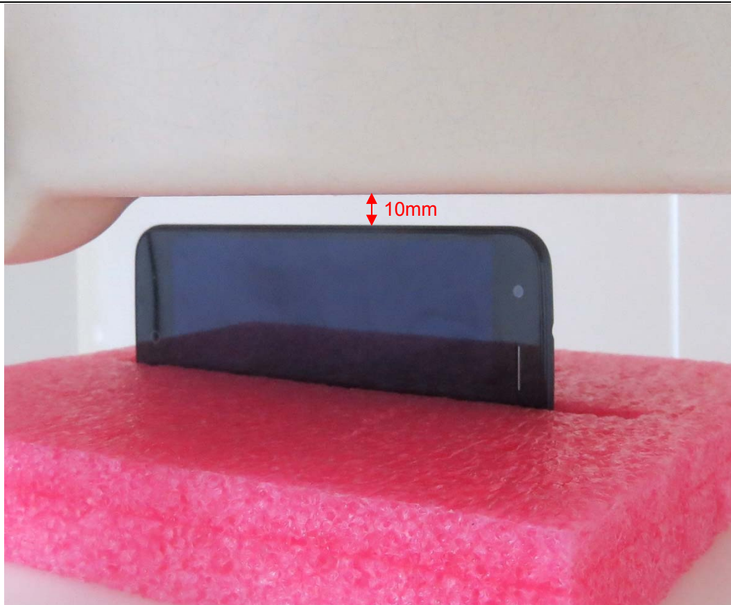
Picture 12: Left Side, the distance from handset to the bottom of the Phantom is 10mm
