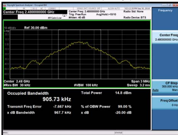
BT DH5 CH78, Carrier frequency (MHz): 2480
