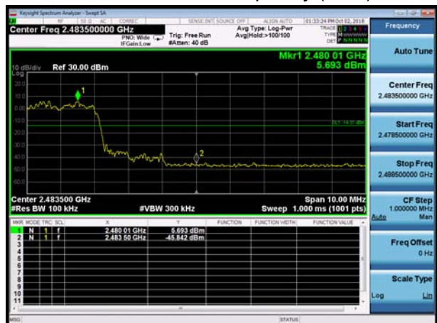
BT 3DH5 CH78, Carrier frequency (MHz): 2480
