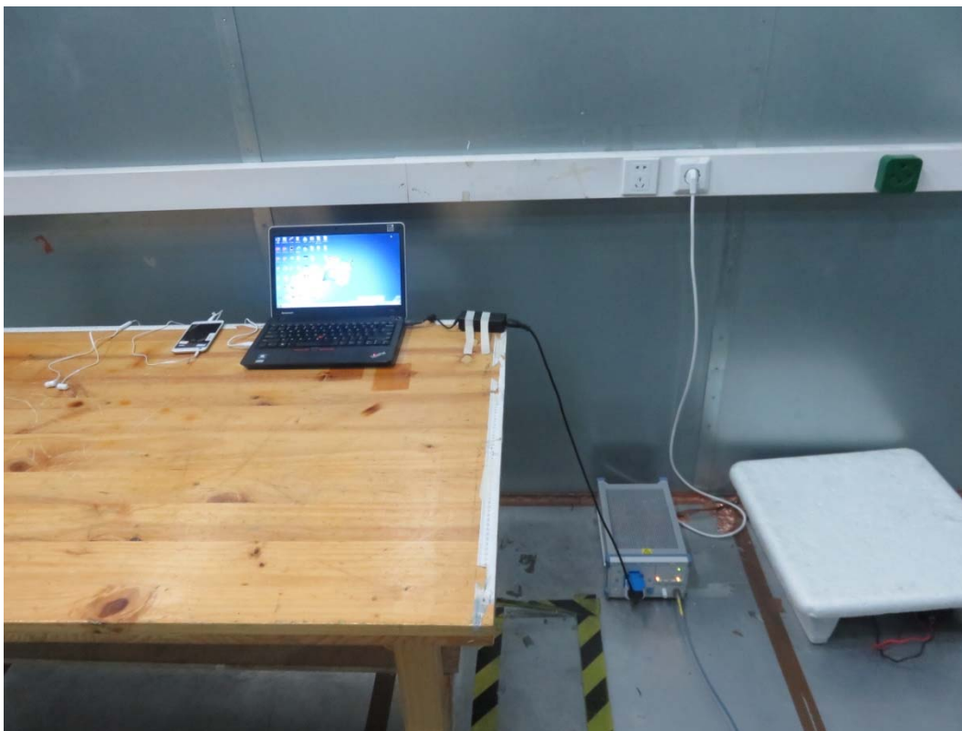
Picture 3 Conducted Emission Test Setup
