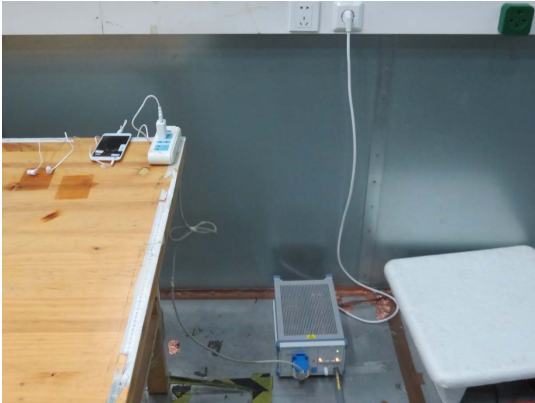
Picture 3 Conducted Emission Test Setup
