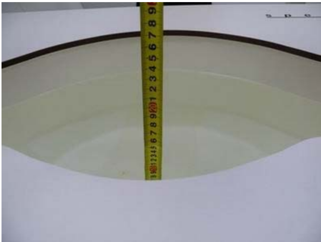
Picture 10: Liquid depth in the flat Phantom (2450 MHz, 15.3cm depth)
