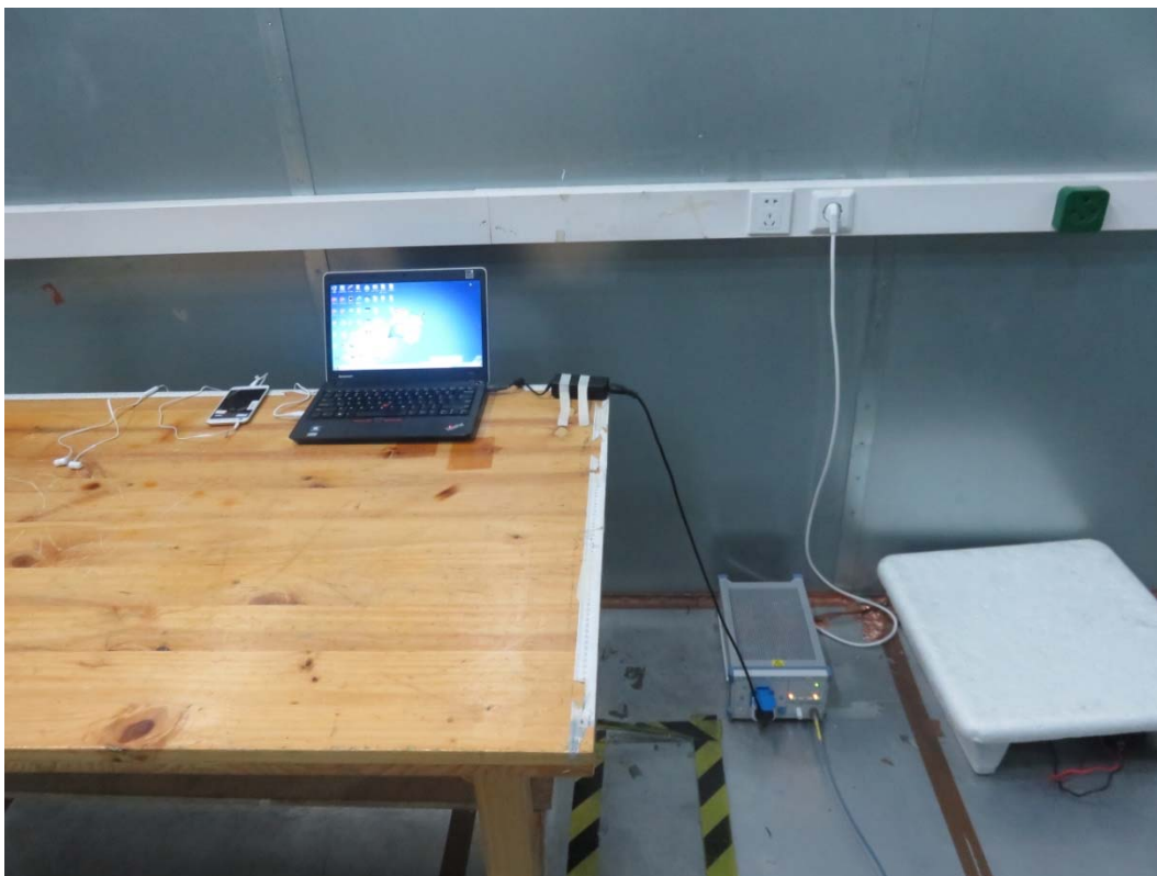
Picture 3 Conducted Emission Test Setup
