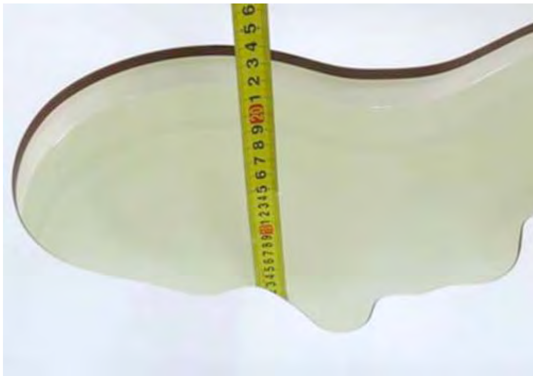
Picture 9: Liquid depth in the head Phantom (2450 MHz, 15.4cm depth)
