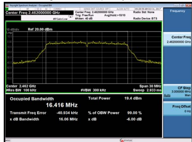
802.11g, Carrier frequency (MHz): 2462
