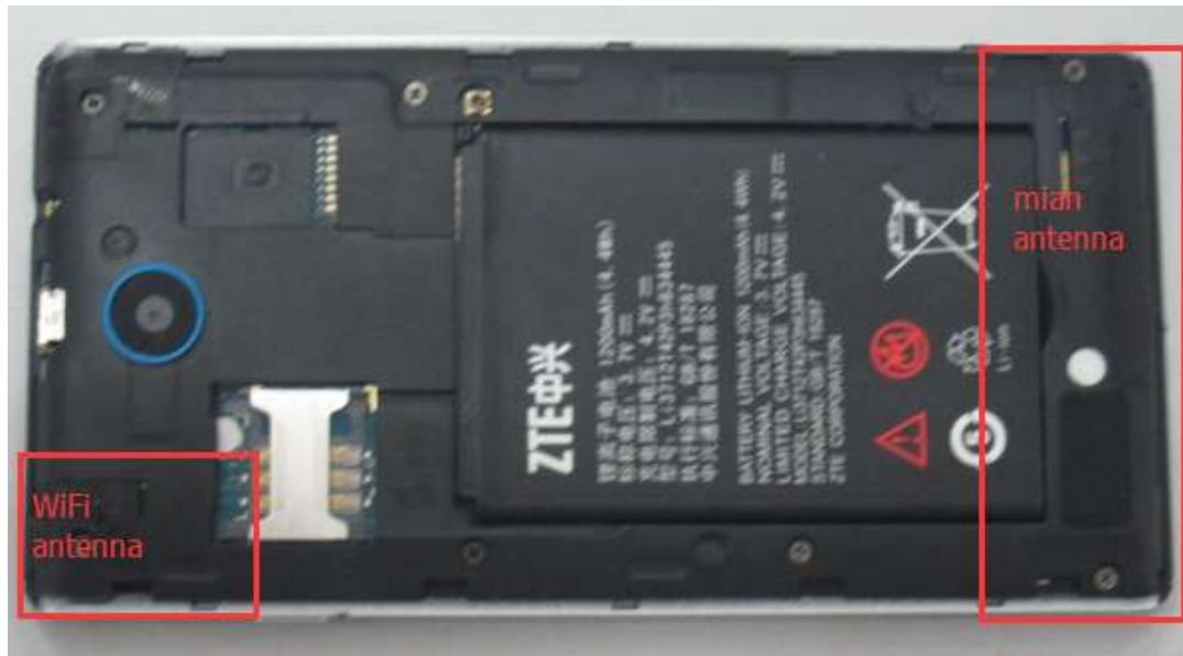
Picture of antennas
