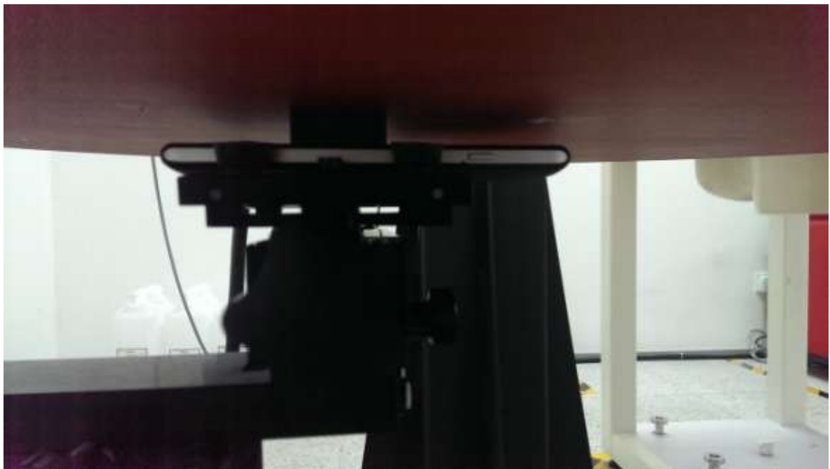
POSITION OF BODY TOWARDS PHANTOM WITH 10mm DISTANCE
