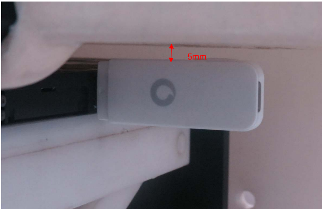
Picture 10: Right Side, the distance from EUT to the bottom of the Phantom is 5mm
