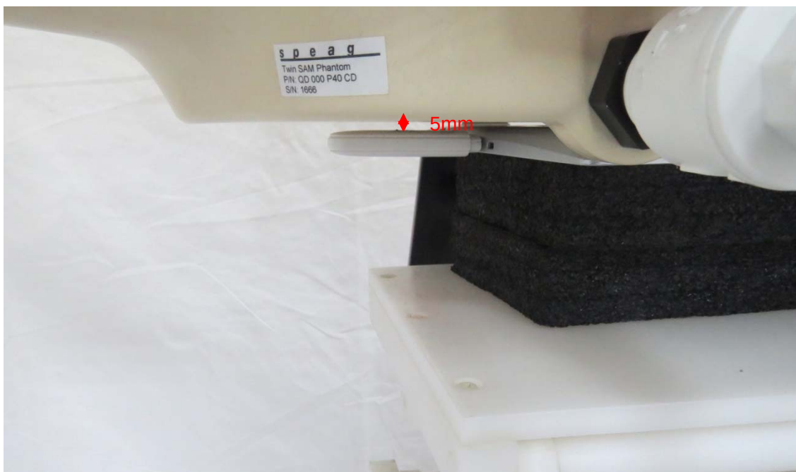
Picture 1: Back Side, the distance from handset to the bottom of the Phantom is 5mm
