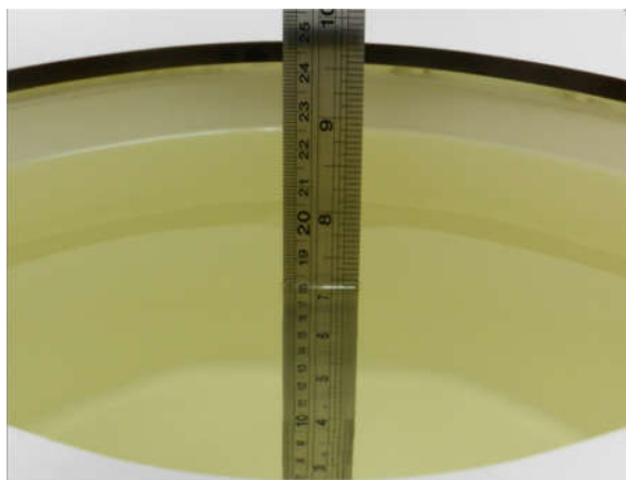
Fig 10.1 Photo of Liquid Height for Body SAR
