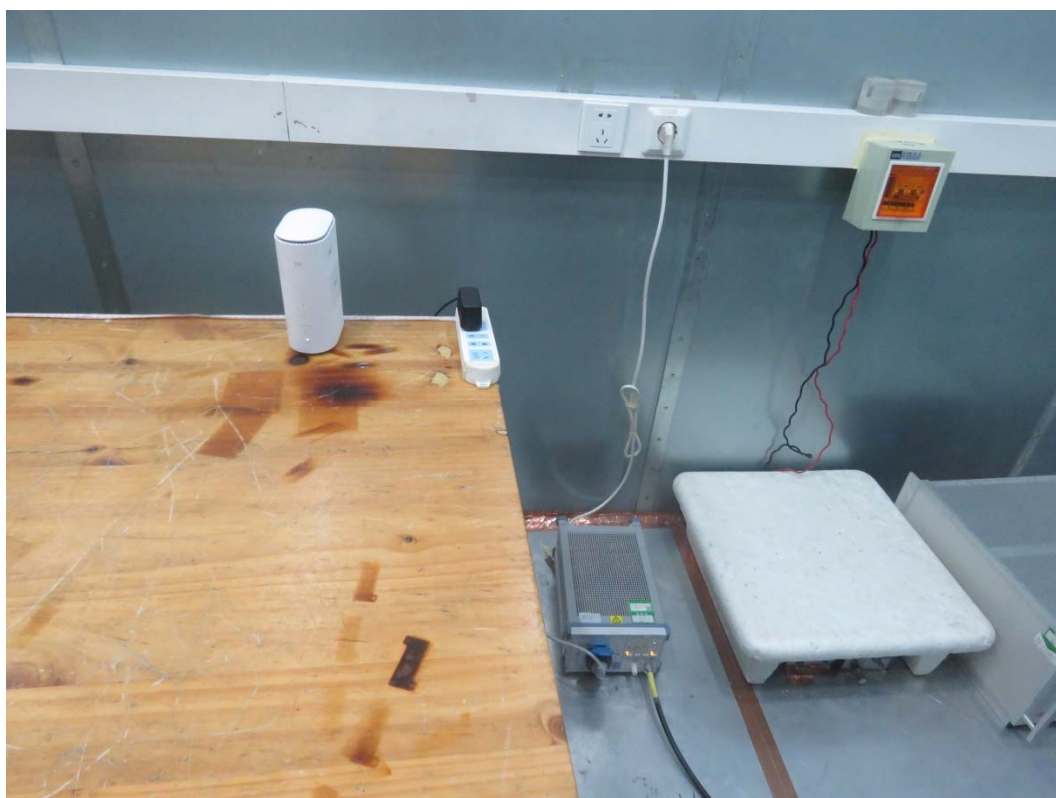
Picture 2 Conducted Emission Test Setup
