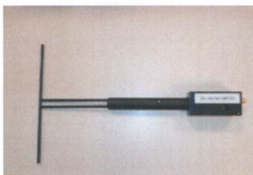
Figure 1 – Satimo COMOSAR Validation Dipole
