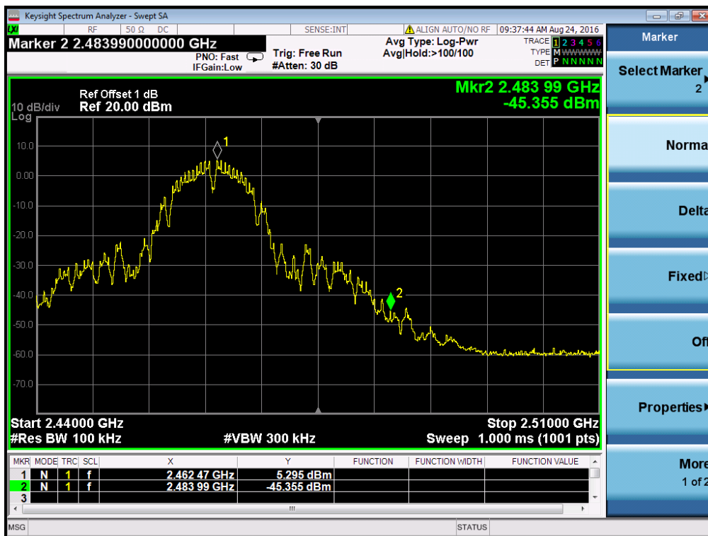
802.11b - High Band Edge Plot on Channel 11
