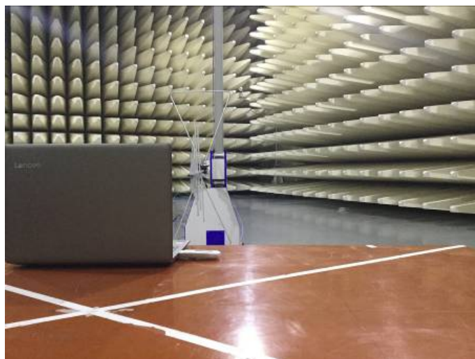
Radiated Emissions Test Setup (with laptop) (30-1000MHz)
