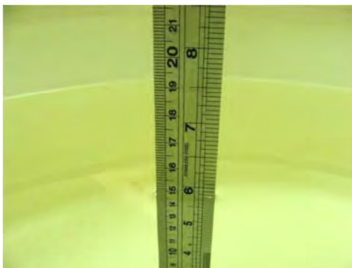
Fig 6.1 Photo of Liquid Height for Body SAR
