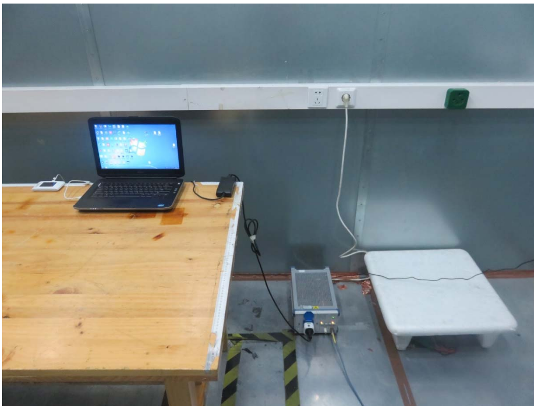
Picture 3 Conducted Emission Test Setup
