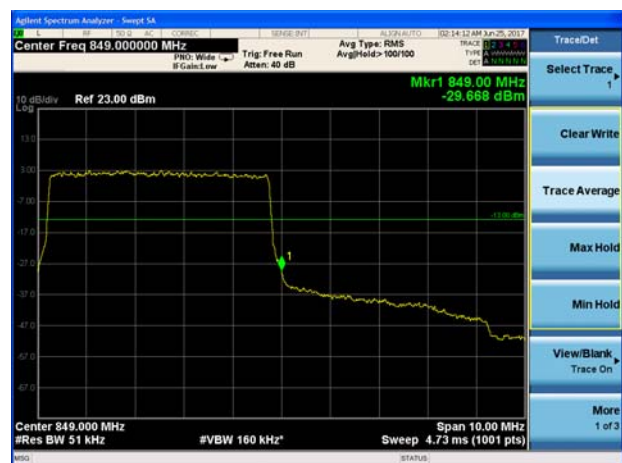
LTE Band 5 QPSK 5MHz CH-High 100%RB
