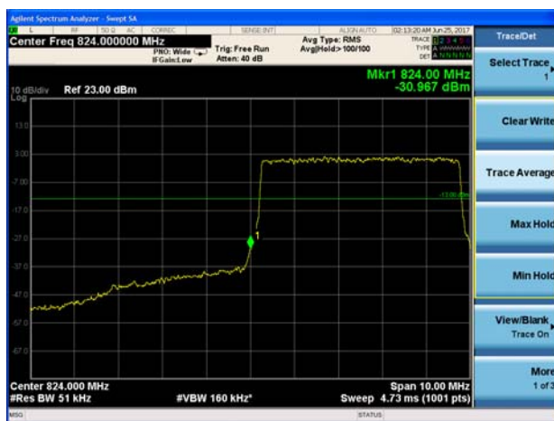
LTE Band 5 16QAM 10MHz CH-Low 1RB
