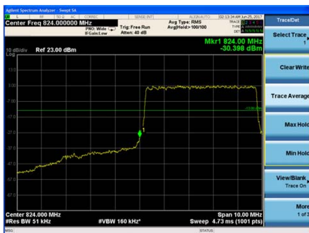
LTE Band 5 QPSK 5MHz CH-Low 100%RB
