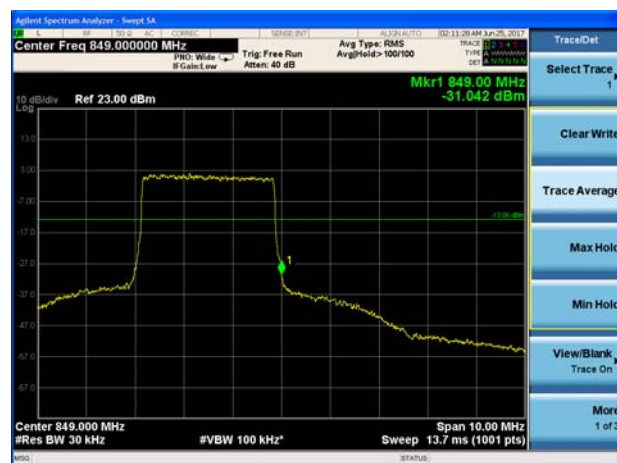
LTE Band 5 16QAM 3MHz CH-High 100%RB
