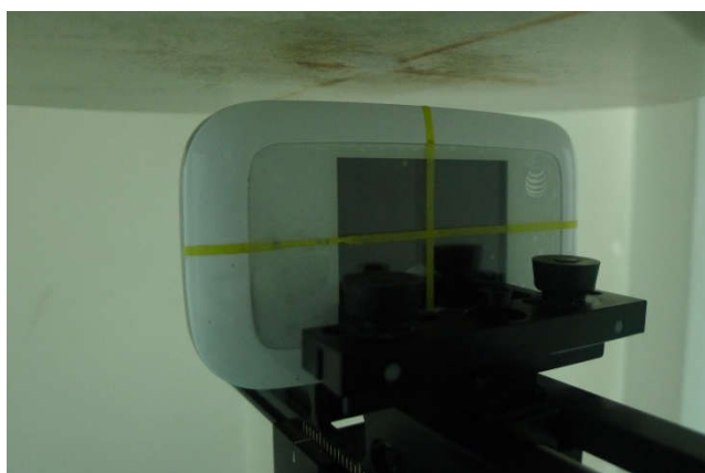
Top Side of, Test Separation 10mm
