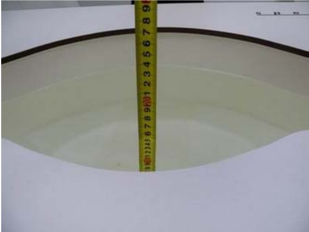
Picture 5: Liquid depth in the flat Phantom (1750 MHz, 15.2cm depth)
