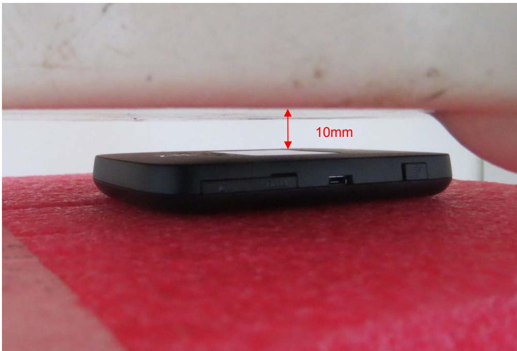
Picture 12: Front Side, the distance from EUT to the bottom of the Phantom is 10mm
