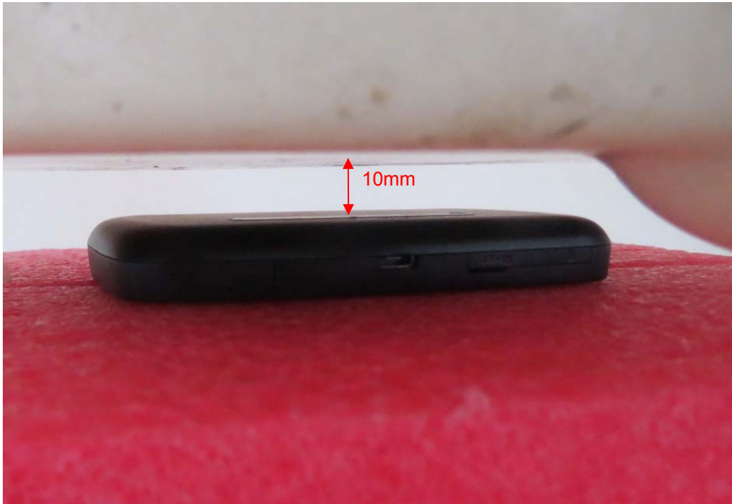
Picture 11: Back Side, the distance from EUT to the bottom of the Phantom is 10mm
