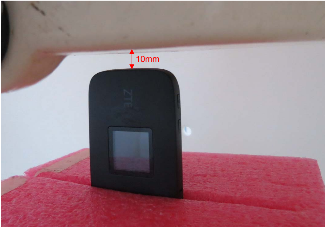
Picture 13: Left Edge, the distance from EUT to the bottom of the Phantom is 10mm
