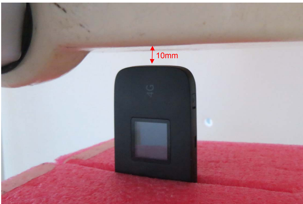
Picture 14: Right Edge, the distance from EUT to the bottom of the Phantom is 10mm
