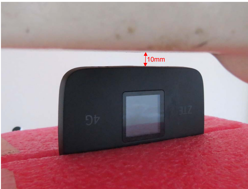
Picture 16: Bottom Edge, the distance from EUT to the bottom of the Phantom is 10mm
