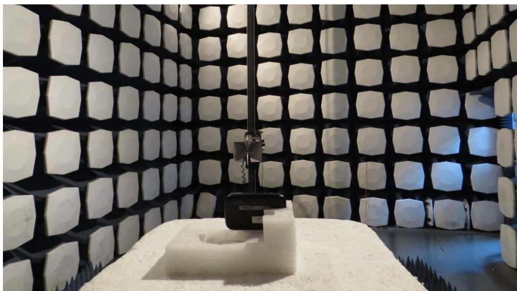
Picture 2: Radiated Spurious Emissions Test setup
