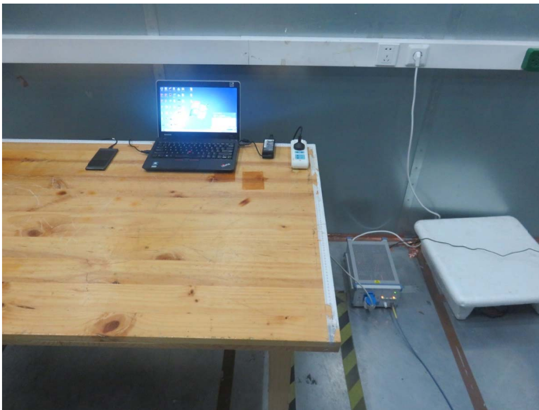
Picture 3 Conducted Emission Test Setup
