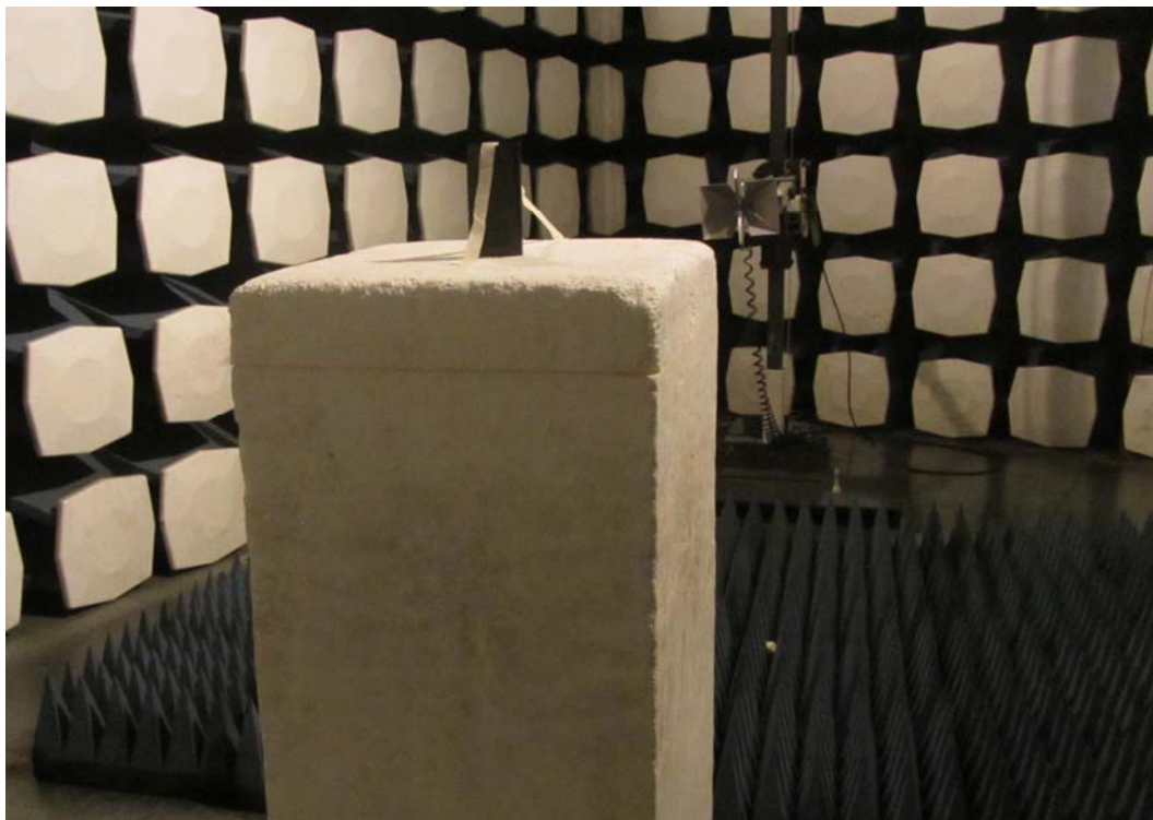
Picture 2: Radiated Spurious Emissions Test setup
