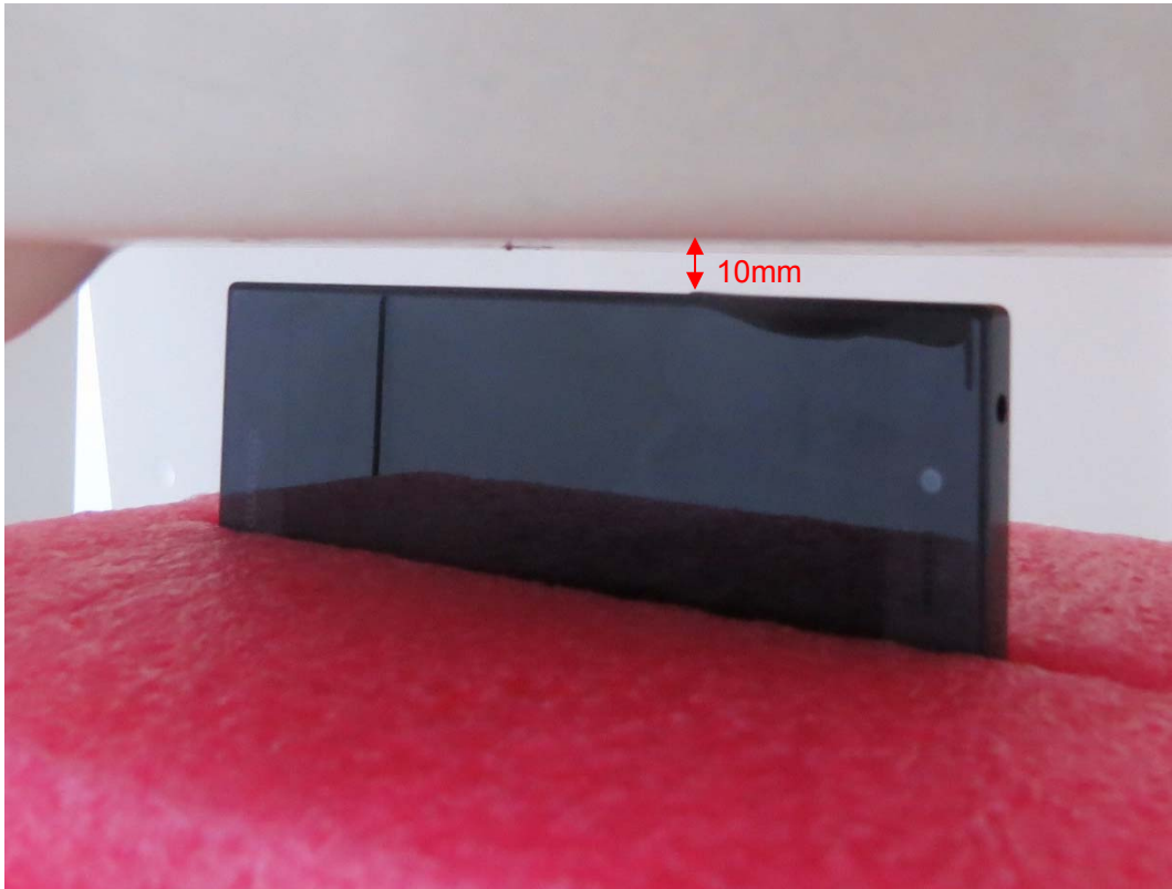
Picture 14: Left Side, the distance from handset to the bottom of the Phantom is 10mm
