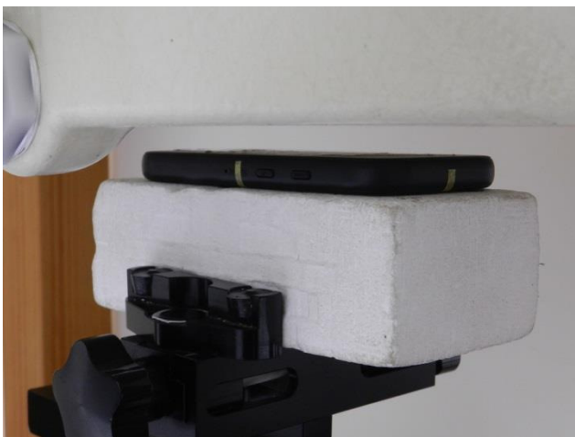
Back, Test Separation 10 mm
