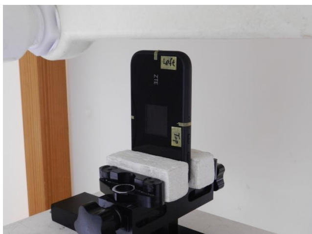
Left Side, Test Separation 10 mm
