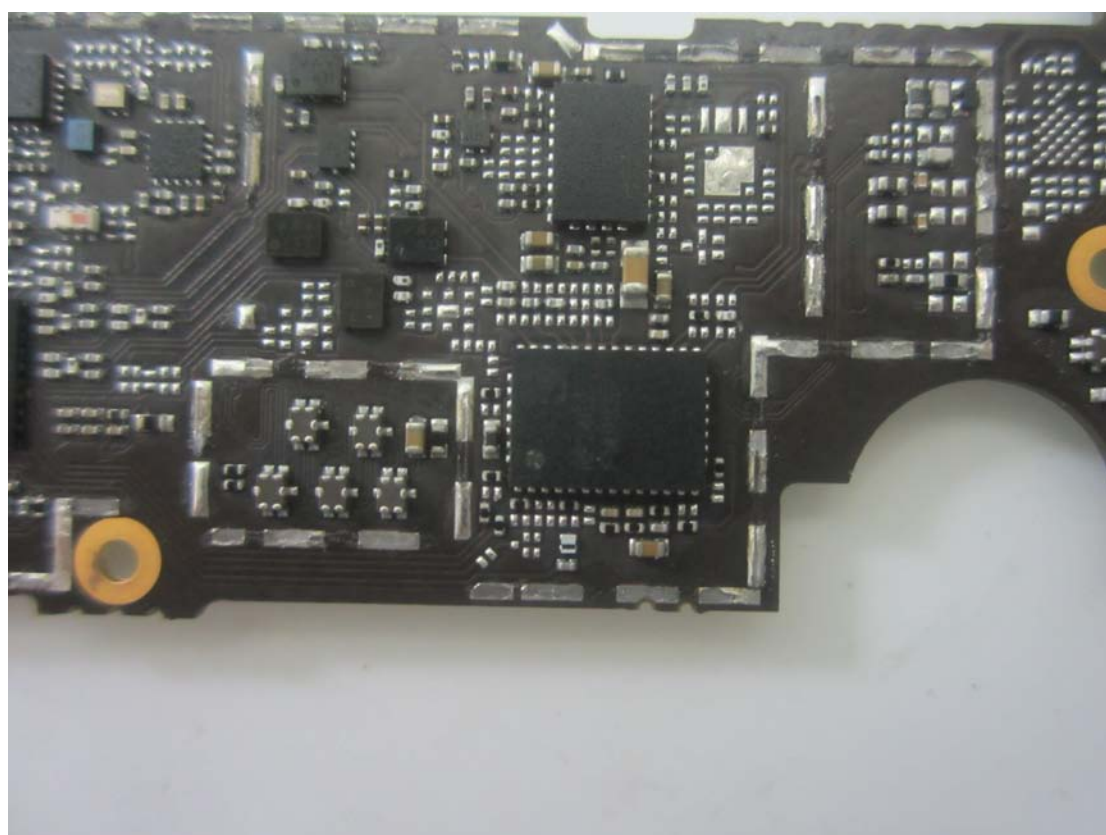
4. GSM/WCDMA/LTE chip view
