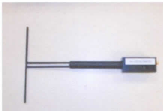
Figure 1 – Satimo COMOSAR Validation Dipole
