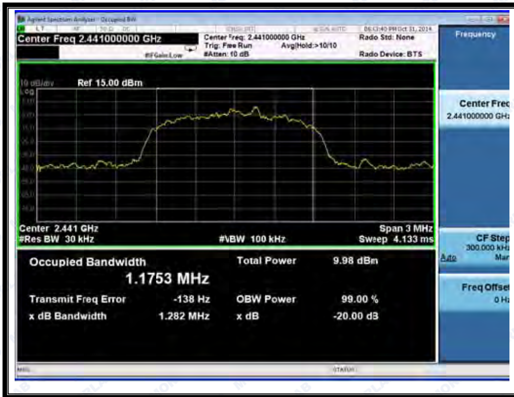
(Plot H: Channel = 2441 @ 8-DPSK)
