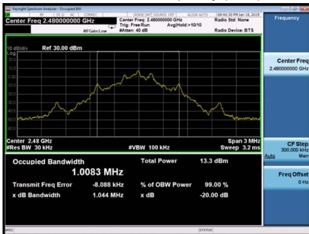
BT DH5 CH78, Carrier frequency (MHz): 2480
