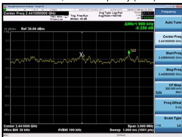
BT 2DH5 CH39, Carrier frequency (MHz): 2441
