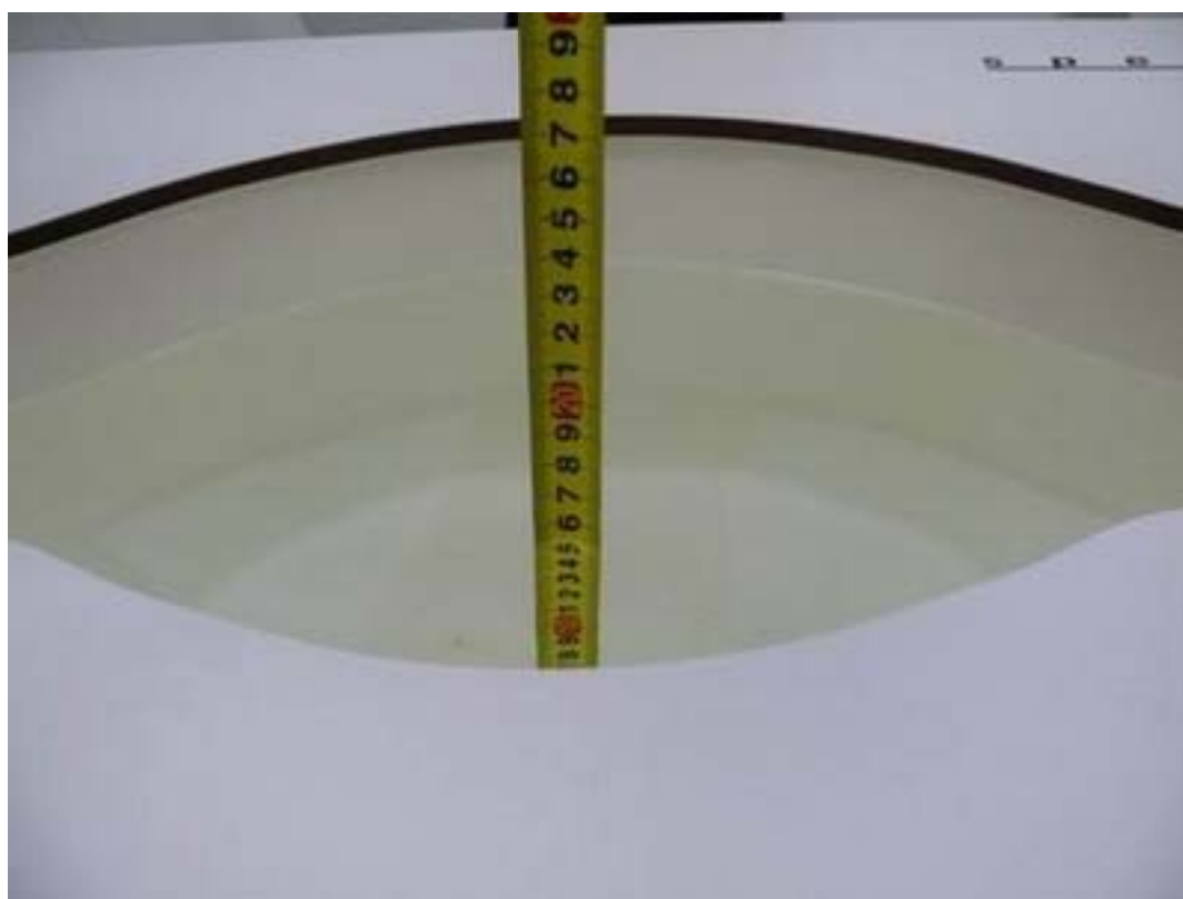
Picture 6: Liquid depth in the flat Phantom (1900 MHz, 15.2cm depth)
