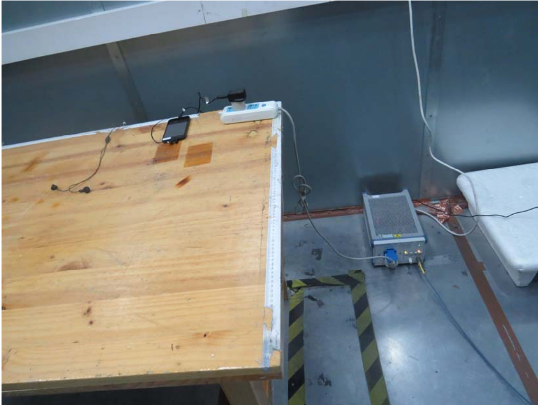
Picture 3 Conducted Emission Test Setup
