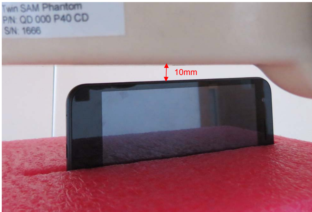
Picture 21: Right Side, the distance from handset to the bottom of the Phantom is 10mm
